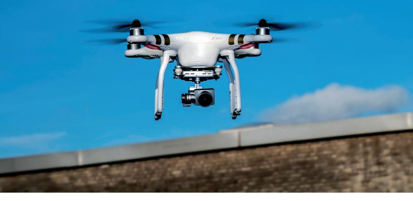
Uniflex® Roof View is an aerial drone-based thermal imaging service that can image entire facilities in a short period of time and in a cost-effective manner. The results can help identify potential wet areas on the roof. Once these spots are identified, the image is reviewed to help determine a course of action.
